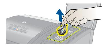
5 Using a soft, dry, lint-free cloth, carefully remove any ink from the contact pads on the printhead and inside the printhead slot in the printer.
